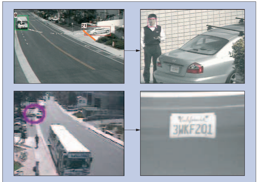
Figure 6. Active camera control. DIVA can define a security zone for intrusion detection, and an event can activate another camera to capture a close-up view.
